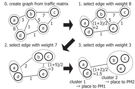
**Fig. 12** An example of the procedures of centralized control with clustering ( $N_C = 2$ ).
