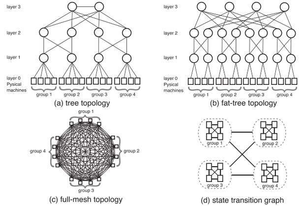
**Fig. 4** Network topologies and state transition graph.
