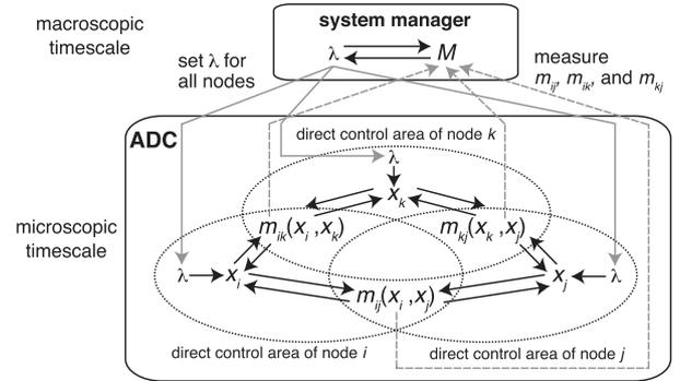
Fig. 3 Multi-timescale control scheme.
