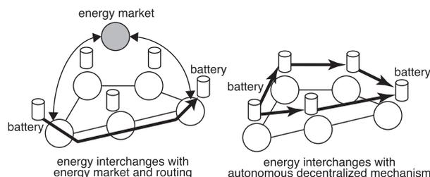
**Fig. 1** Energy interchanges with energy market and routing (left) and autonomous decentralized mechanism (right).
