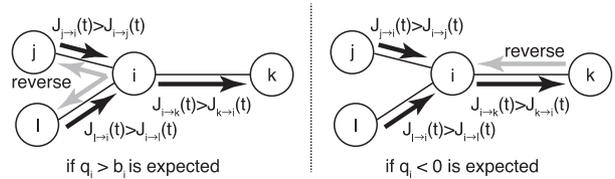
**Fig. 4** Procedure for preventing the overrun and underrun of node energy  $q_i(t)$ .
