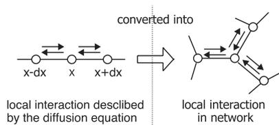
**Fig. 2** The conversion from the local interaction described in the diffusion equation to the local interaction in a network.
