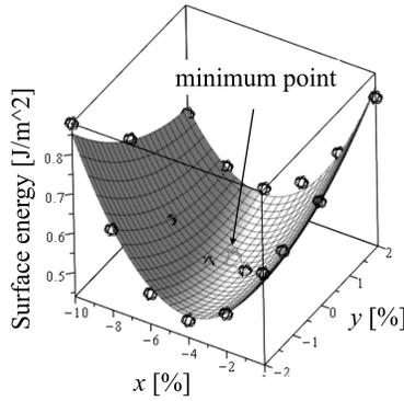
Figure 3: Energy surface of unit cell dimension changes.
