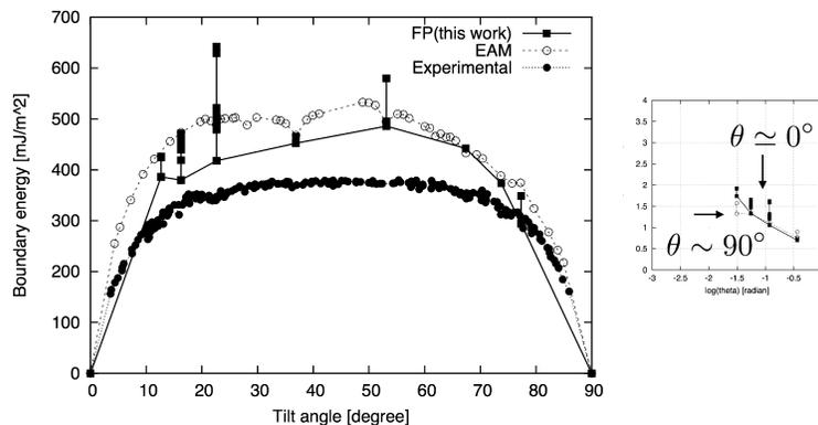
Figure 5: Tilt angle dependency of the boundary energy on Al  $\langle 100 \rangle$  direction obtained by the first principles calculations. Experimental and EAM calculated results are also plotted. The right hand panel shows the  $E/\theta - \log \theta$  plot. See text for details.
