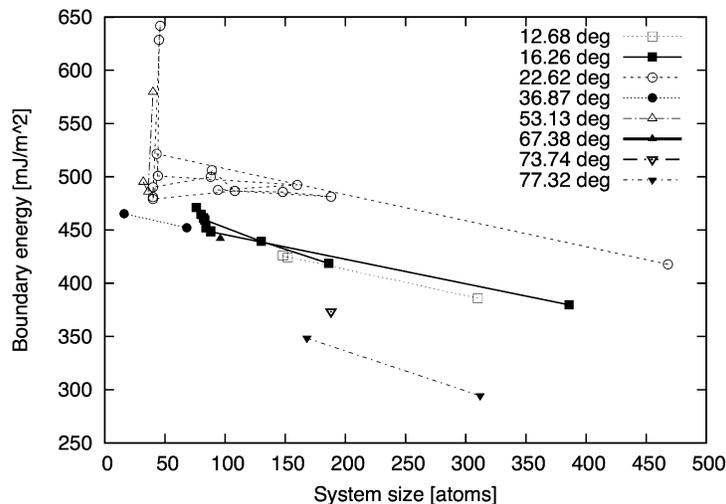
Figure 4: Size dependency of boundary energy for each tilt angle.
