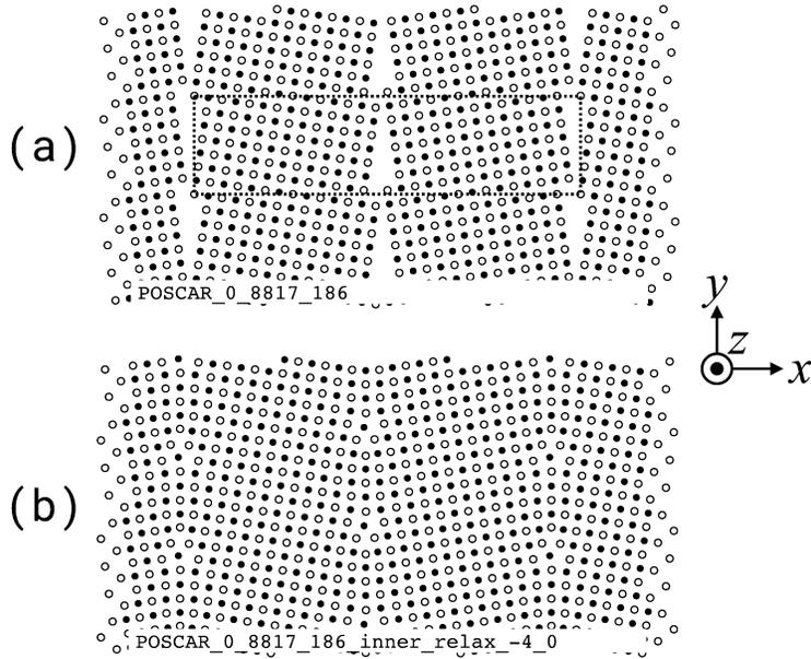
Figure 2: Top views of the boundary model for the misorientation angle of  $12.26^\circ$ , (a) before and (b) after relaxations.
