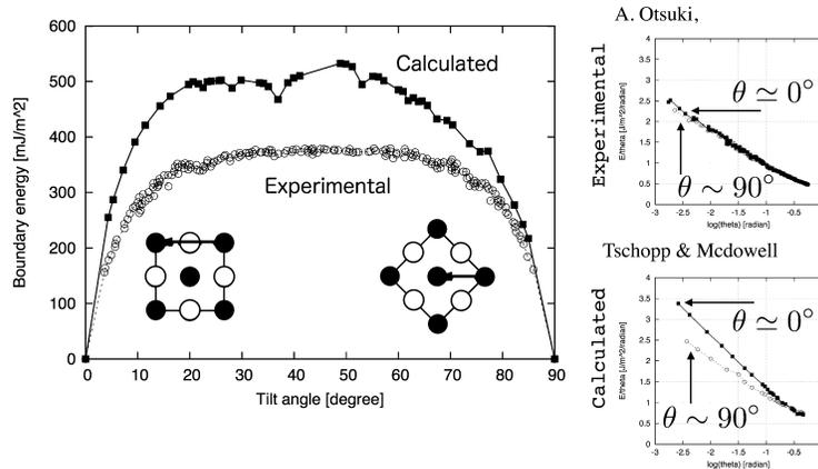
Figure 1: Experimental and calculated  $\theta$  dependency of symmetric tilt grain boundary energy of Al. See text for details.
