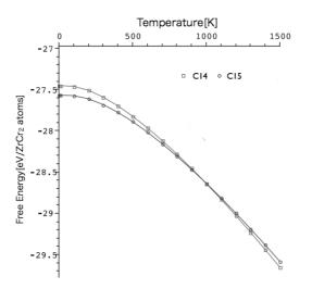
Fig.1 Temperature dependency of vibration free energy change of ZrCr<sub>2</sub> Laves phases.
