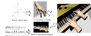
Figure 1: Process of making CG animation of piano performance, and an example scene.
