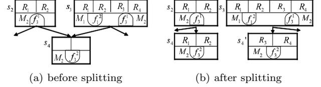
**Figure 7:** State splitting by register binding.
