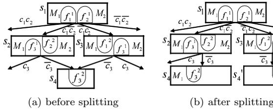
**Figure 6:** State splitting by operation binding.
